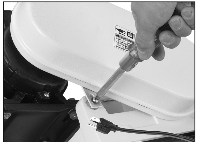
Figure 10. Installing pulley cover.
